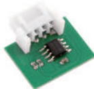
250SM1022 Memory card for 1022 radio codes
