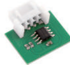
250SM126 Memory card for 126 radio codes
