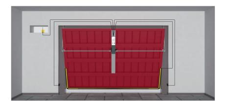
The above represented installation does not include safety devices such as safety edges. Their addition depends upon the risk assessment made on any installation in accordance with EN 12453 standards.
